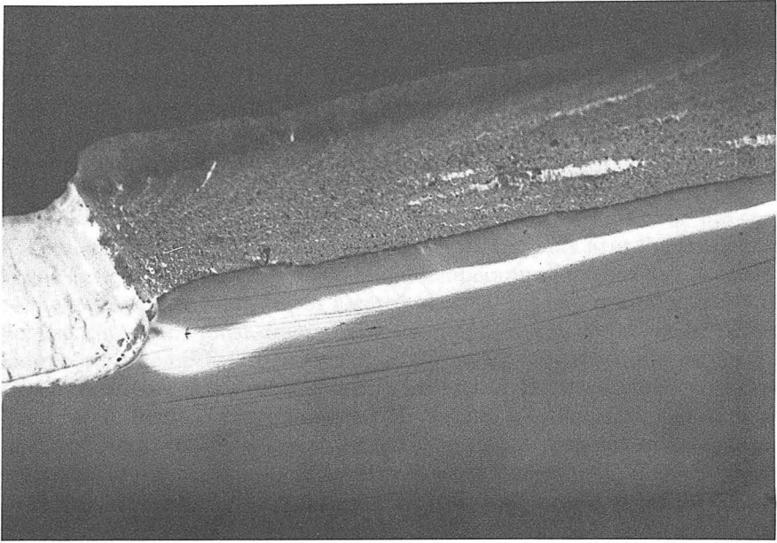
Figure 5.25. Photograph of fracture surface and shear lips.
