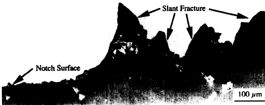
Figure 6. Optical micrograph of the crack profile from the mating half of metallic glass specimen shown in Fig. 5. Regions of both slant fracture and flat fracture are observed. The initial notch is on the left of the micrograph.
