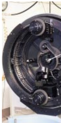
Above: A peek inside the 2-million-frame-per-second camera, which—believe it or not—uses ordinary 35-millimeter film. The arrow points to the rotating three-sided mirror, which bounces the light off a nest of other mirrors before it finally reaches the film at the periphery—you can see the laser's green dot there. Both cameras were manufactured by the Cordin Company of Salt Lake City, Utah.
