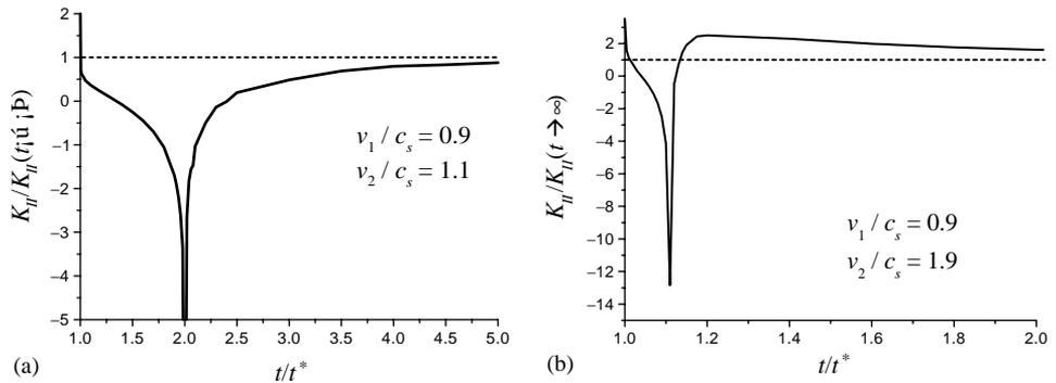
Fig. 4. The stress intensity factor,  $K_{II}$ , normalized by  $K_{II}(t \rightarrow \infty)$ , around a crack tip that suddenly accelerates from a sub-Rayleigh velocity,  $v_1$ , to an intersonic velocity,  $v_2$ . Time  $t$  is normalized by the crack propagation time  $t^*$ ; Poisson's ratio  $\nu = \frac{1}{3}$ . The initial velocity is  $v_1 = 0.9c_s$ , and is accelerated to (a)  $v_2 = 1.1c_s$  and (b)  $v_2 = 1.9c_s$ .
