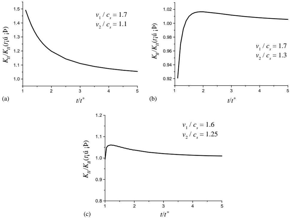
Fig. 2. The stress intensity factor,  $K_{II}$ , normalized by  $K_{II}(t \rightarrow \infty)$ , around a crack tip that suddenly decelerates from an intersonic velocity,  $v_1$ , to a another intersonic velocity,  $v_2$ . Time  $t$  is normalized by the crack propagation time  $t^*$ ; Poisson’s ratio  $\nu = \frac{1}{3}$ . The crack tip velocities are (a)  $v_1 = 1.7c_s$ ,  $v_2 = 1.1c_s$ ; (b)  $v_1 = 1.7c_s$ ,  $v_2 = 1.3c_s$ ; (c)  $v_1 = 1.6c_s$ ,  $v_2 = 1.25c_s$ .
