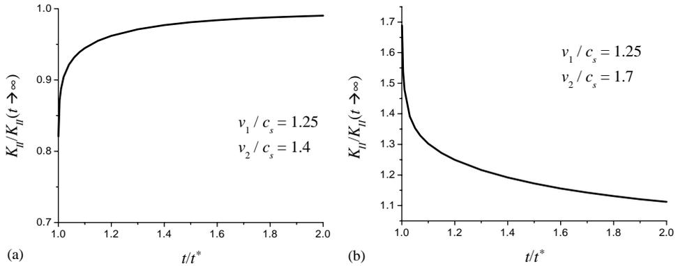
Fig. 3. The stress intensity factor,  $K_{II}$ , normalized by  $K_{II}(t \rightarrow \infty)$ , around a crack tip that suddenly accelerates from an intersonic velocity,  $v_1$ , to another intersonic velocity,  $v_2$ . Time  $t$  is normalized by the crack propagation time  $t^*$ ; Poisson's ratio  $\nu = \frac{1}{3}$ . The initial crack tip velocity is  $v_1 = 1.25c_s$ , the crack is suddenly accelerated to (a)  $v_2 = 1.4c_s$  and (b)  $v_2 = 1.7c_s$ .
