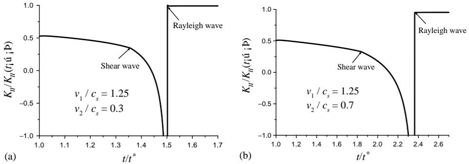
Fig. 1. The stress intensity factor,  $K_{II}$ , normalized by  $K_{II}(t \rightarrow \infty)$ , around a crack tip that suddenly decelerates from an intersonic velocity,  $v_1$ , to a sub-Rayleigh velocity,  $v_2$ . Time  $t$  is normalized by the crack propagation time  $t^*$ ; Poisson’s ratio  $\nu = \frac{1}{3}$ . The initial crack tip velocity is  $v_1 = 1.25c_s$ , and is decelerated to (a)  $v_2 = 0.3c_s$  and (b)  $v_2 = 0.7c_s$ .
