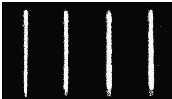
Fig. 14. COD profiles at (left to right) 20, 164, 326, and 344 \mu s for a 6Al-4V Ti specimen (no side-grooves) impacted at 3 m/s (initial notch length visible = 12.71 mm). Note that digital image processing is required to extract meaningful data.
