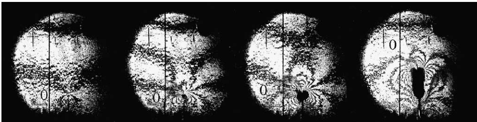
Fig. 18. CGS fringe patterns at (left to right) 3, 38, 78, and 138 \mu s for a 6Al-4V Ti specimen impacted at 9 m/s (beam diameter = 50 mm).
