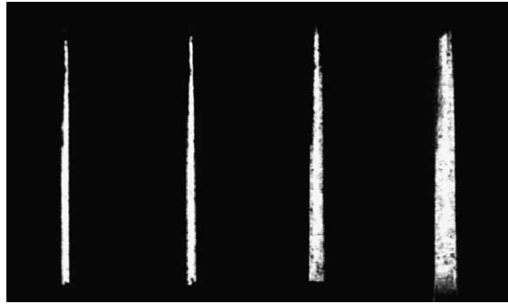
Fig. 19. COD profiles at (left to right) 6, 38, 78, and 142 \mu s for a 6Al–4V Ti specimen (no side-grooves) impacted at 9 m/s (initial notch length visible = 10.82 mm).
