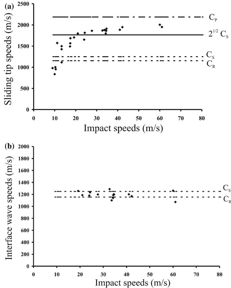
Figure 8. (a) Variation of the sliding tip speed with the impact speed. The confining stress was 10 MPa. (b) The wrinkle-like pulse speed remained between the Rayleigh wave speed and the shear wave speed of Homalite-100, independent of the impact speed.
