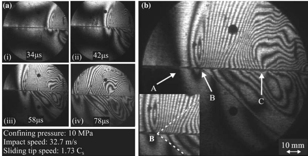
Figure 3. (a) Isochromatic fringes of intersonic sliding propagation at different time instances. (b) The  $p$ -wave front (A), the sliding tip (B), and the detachment interface wave (C) are shown clearly in the magnification of the fringe pattern (iii).
