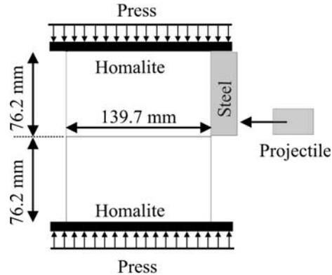
Figure 1. Geometry and loading configuration for a specimen constituted by two identical incoherent plates.
