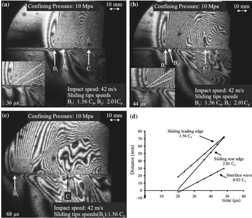
Figure 5. (a–c) Isochromatic fringes of sliding propagation at different time instances. Two sliding tips ( $B_1$  and  $B_2$ ) were propagating at different intersonic speeds. In the inserts the dual and single Mach lines are marked. (d) Positions of the sliding leading edge, the second sliding tip and the detachment interface wave as a function of time.
