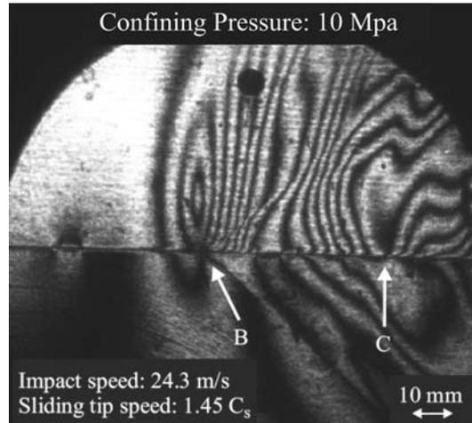
Figure 6. Isochromatic fringes of sliding propagation.
