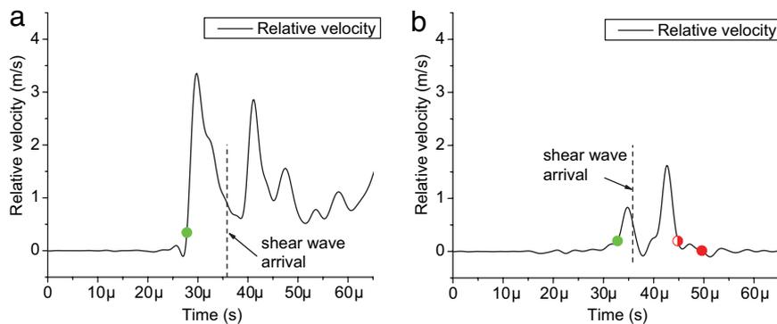
**Fig. 4.** Relative velocity records, at 40 mm away from the hypocenter, that capture the sub-Rayleigh to supershear transition. (a) A sub-Rayleigh crack transitioning to a supershear crack ( $\alpha = 30^\circ$ ,  $P = 14$  MPa). (b) A sub-Rayleigh pulse transitioning to a supershear pulse ( $\alpha = 27.5^\circ$ ,  $P = 14$  MPa).
