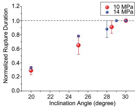
**Fig. 3.** Rupture duration, normalized by the maximum potential sliding time, plotted as a function of inclination angle  $\alpha$  for two values of far-field pressure  $P$ . Normalized rupture duration of 1 corresponds to crack-like ruptures, whereas smaller values correspond to progressively narrower pulse-like ruptures.
