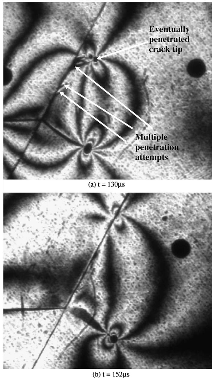
Fig. 13. Details of deflected crack of both specimen configurations for  $\alpha = 60^\circ$ .
