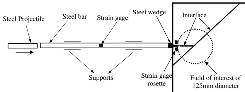
Fig. 2. Modified Hopkinson bar loading setup.
