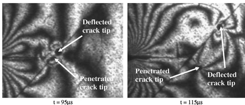
Fig. 10. Sequence of frames showing slight delay of penetrated crack compared to deflected crack for the specimen configuration shown in Fig. 8a.
