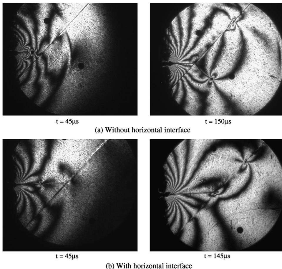
Fig. 8. Isochromatics associated with propagating crack for an inclined interface,  $\alpha = 45^\circ$ .
