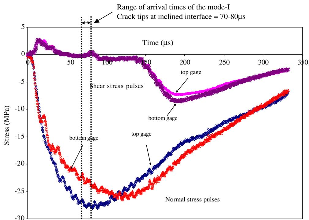
Fig. 3. Typical normal and shear loading pulses.
