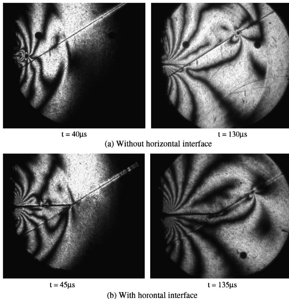
Fig. 5. Isochromatics associated with a propagating crack for an inclined interface,  $\alpha = 30^\circ$  (the black circular spot in the figures represents a scale of 6.25 mm).
