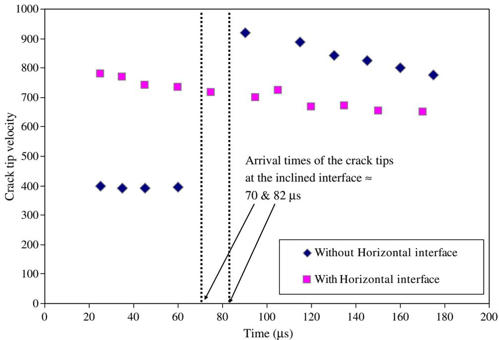
Fig. 9. Crack tip velocity history of a propagating crack for an inclined interface,  $\alpha = 45^\circ$ .
