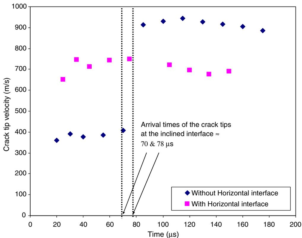
Fig. 6. Crack tip velocity history of a propagating crack for an inclined interface,  $\alpha = 30^\circ$ .
