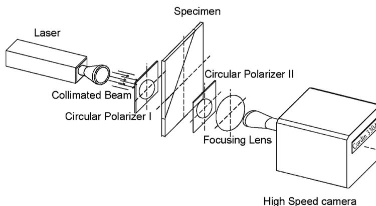
Fig. 4. Dynamic Photoelastic experimental setup.
