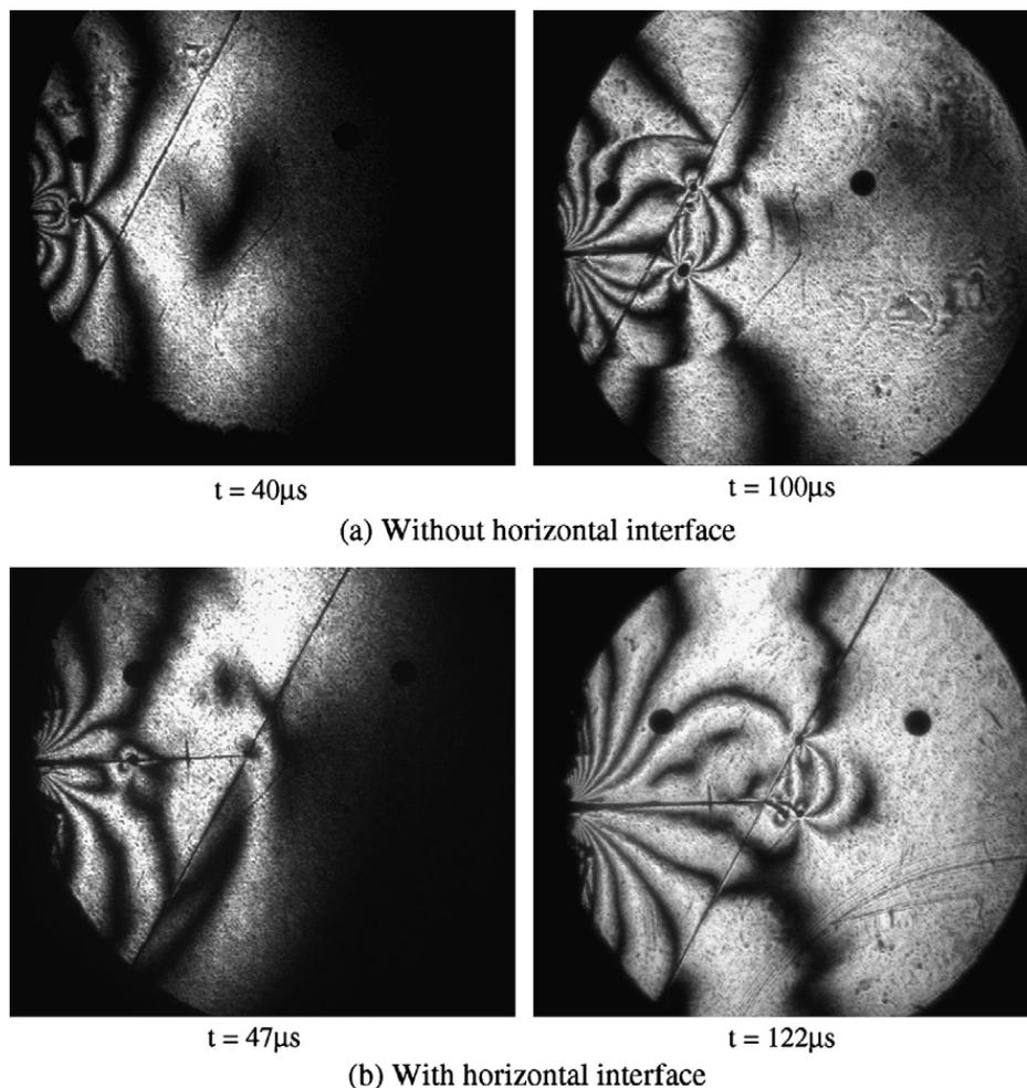
Fig. 11. Isochromatics associated with propagating cracks for an inclined interface,  $\alpha = 60^\circ$ .
