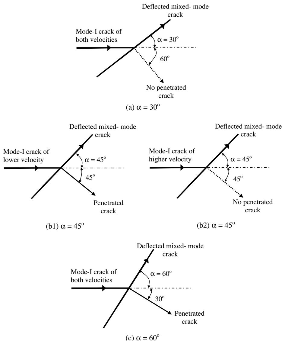
Fig. 7. Schematic diagram showing the deflection/penetration behavior of incoming mode-I crack when it reaches inclined interface.
