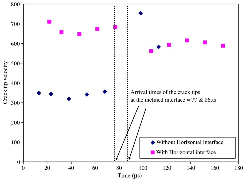
Fig. 12. Crack tip velocity history of a propagating crack for an inclined interface,  $\alpha = 60^\circ$ .
